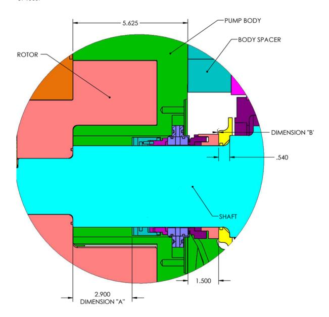
2) See table below to determine proper seal setting for inner and outer seal. Due to the seal setting flexibility, the seal setting is calculated in .015" increments.
